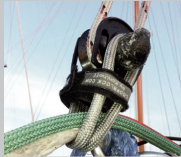
2:1 Main Halyard Block LB60-3 on a JV52 after three years of use.
