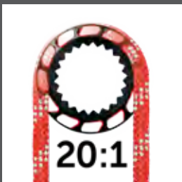
Ratchet block holding power
