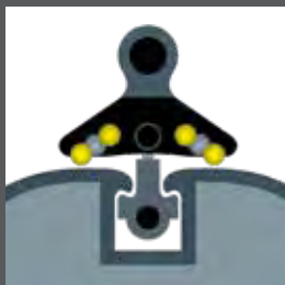
Use existing mast luff groove
