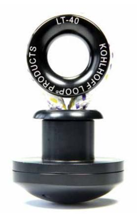
KOHLHOFF LOOP® Padeyes are through-deck fittings made of hard anodised aluminium. Both parts are screwed together to provide easy adjustment for different deck thicknesses. They are all fully water tight with an Acetal cover encapsulating the dogbone and loop on the underside of the fitting. KOHLHOFF LOOP® Padeyes come in black as standard but are also available in silver on request.
