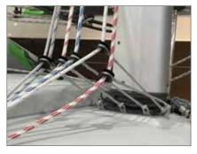
LOOP® Strops to adjust the right hight for halyard deflection
